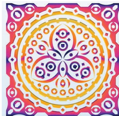
5. Shown is the electric-field distribution on the unit cell of the frequency-selective surface at 1.9 GHz.
